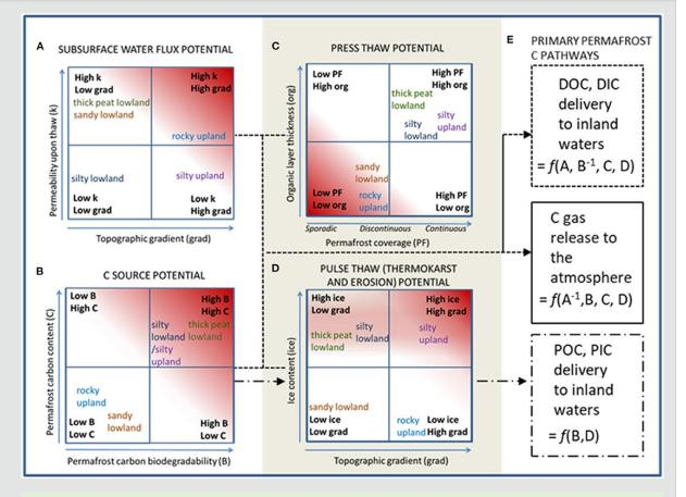
Consideration of competing hydrologic, biogeochemical, and physical influences is required to determine the fate of permafrost carbon (E). Red shading in panels represents conditions having the highest potential for (A) subsurface water flux, (B) carbon source strength, (C) press thaw, and (D) pulse thaw.
